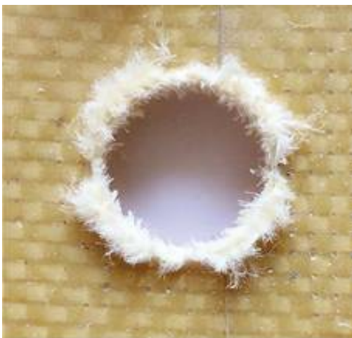
Fig. 5 Uncut fibers created in Kevlar/epoxy composite drilling
