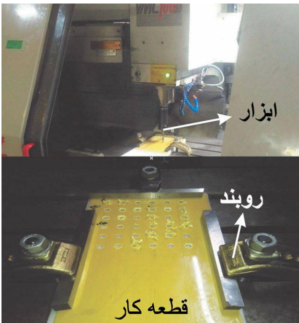
Fig. 2 Experimental tests implementation and composite sheet clamping
