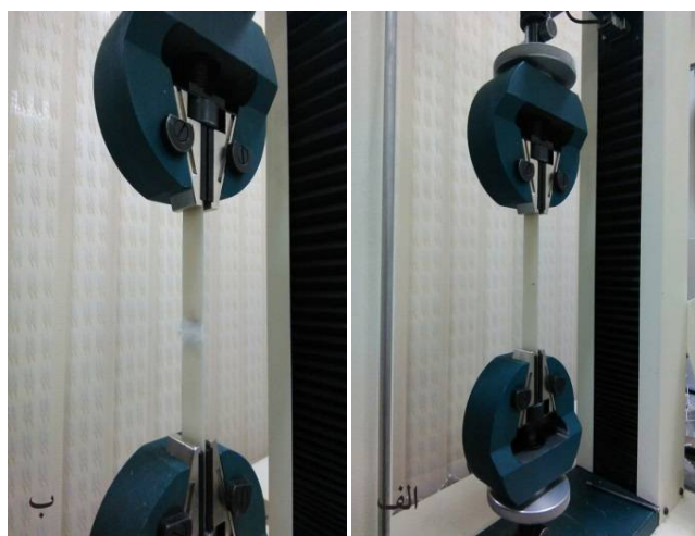
Fig. 2 Tensile test procedure, a) at the moment and b) at the end of test until sample's fracture
