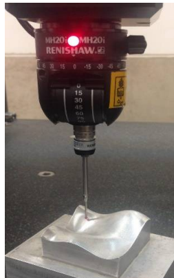
Fig.2 Sampling from a free-form surface to extract the machining model
