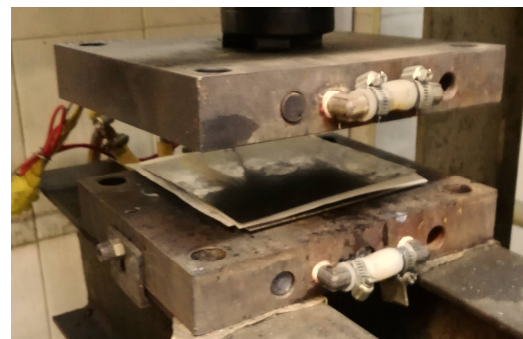
Fig. 2 Forming the PU/PCL blend with hot press set-up
