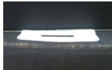
Fig. 12 Hollow rectangular side view to measure distortion
