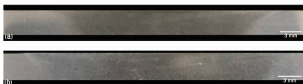
Fig. 2 Cross section macrostructure of processed specimens, a) FS and b) FSV processed specimens
