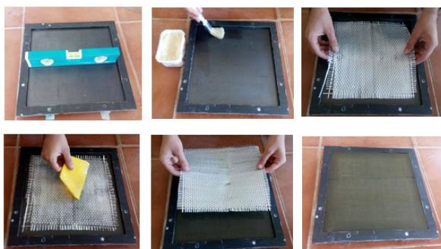
Fig. 1 Hand-layup method for composite samples
