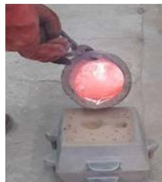
Fig. 5 Molten metal cast and vaporizes foam pattern
