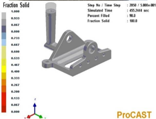
Fig. 8 Result of casting and simulation in ABS part.
