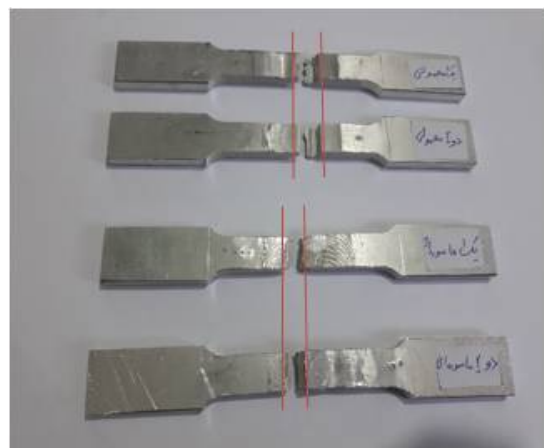
Fig. 8 The fractured samples under the tensile test
