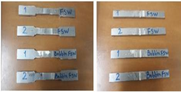
Fig. 4 The prepared samples for the tensile and Charpy impact tests
