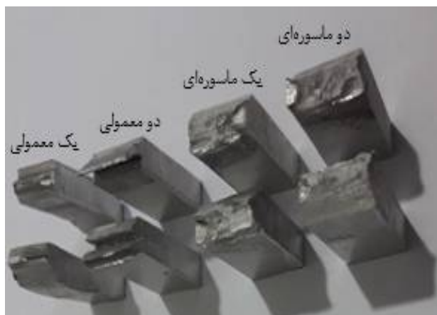
Fig. 10 The fractured samples under the Charpy impact test
