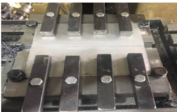
Fig. 3 The welding samples in the fixture
