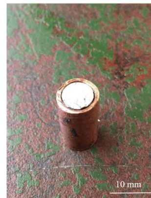
Fig. 1 Two-layer rod for hot forward extrusion
