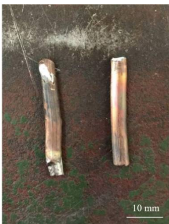
Fig. 5 Hot forward extruded Al-Cu rods
