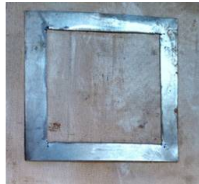
Fig. 1 Applied steel mold with the dimensions of 150×150×1 mm
