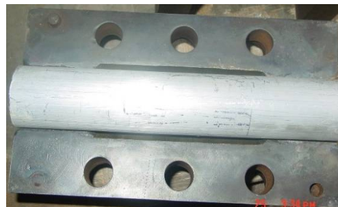
Fig. 4 No deformation with initial gas pressure of 6bar
