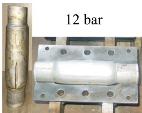
Fig. 6 Tube deformation under initial gas pressure of 12bar with ignition system at the end of tube
