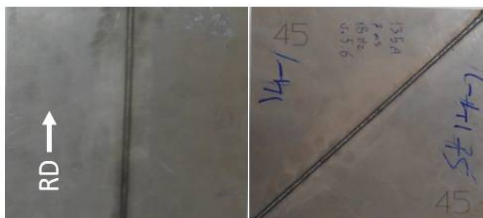
Fig. 5 The samples prepared in two directions of welding line line
