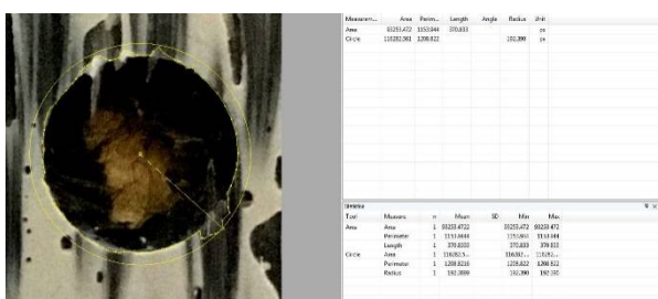
Fig. 8 Image processing for 3 mm CFRP with 10mm drilling diameter and a feed rate of 80 mm/min
