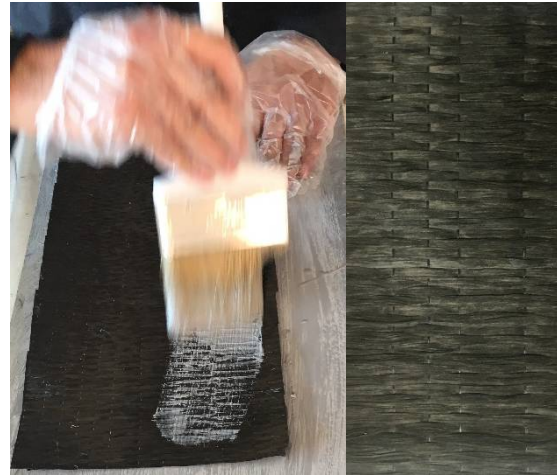
Fig. 2 Hand layup for manufacturing CFRP
