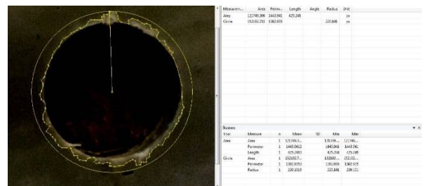
Fig. 12 Image processing for 4 mm CFRP with 10mm drilling diameter and a feed rate of 125 mm/min
