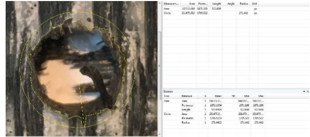
Fig. 9 Image processing for 4 mm CFRP with 10mm drilling diameter and a feed rate of 630 mm/min
