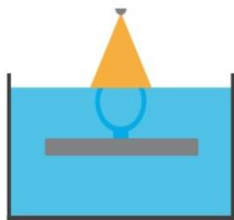
Fig. 1 The reason for the need to control the depth of light penetration to keep the areas in the arc (pale areas) fluid while curing the wall and the hollow part's roof (bold areas).
