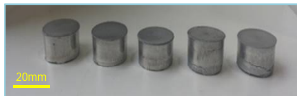
Fig. 4 Fabricated samples by dynamic compaction method
