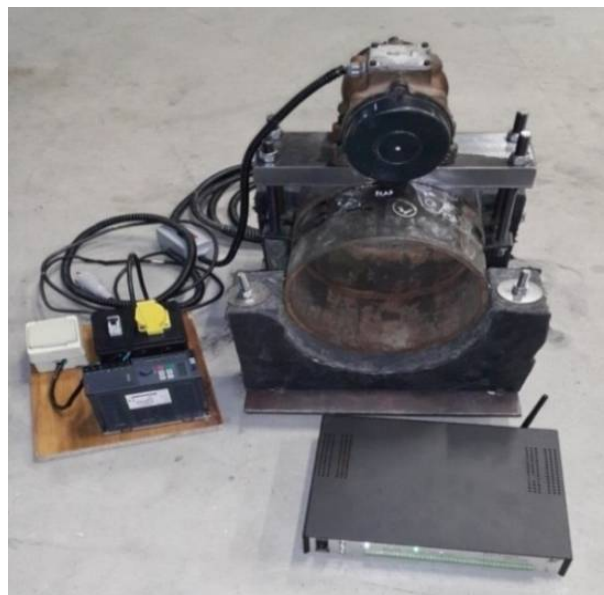
Fig. 3 Vibration stress relief setup on pipe
