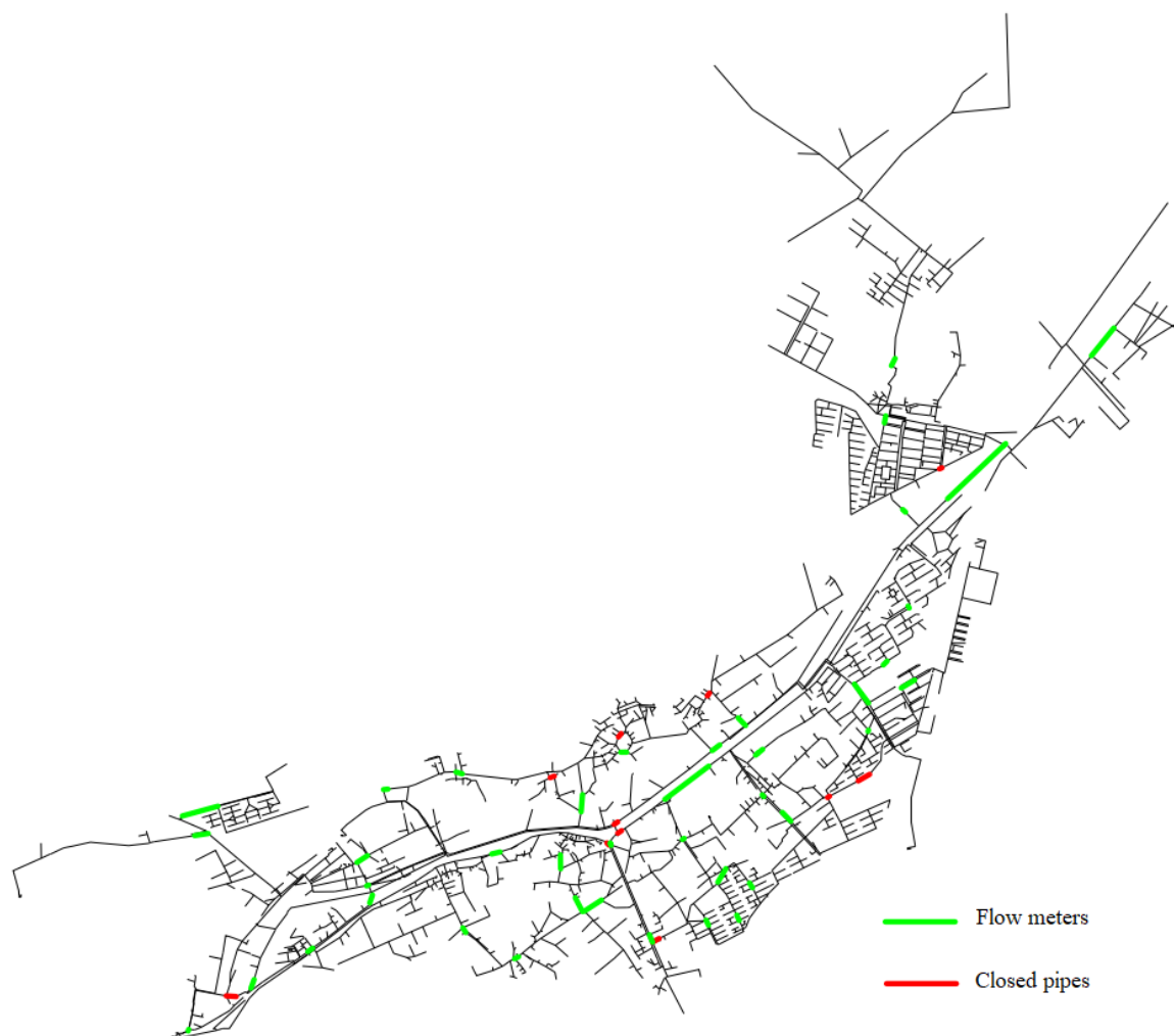
Fig. 4- Boundary pipes optimization results
