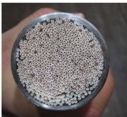
Fig. 2. Propylene membrane used in the system
