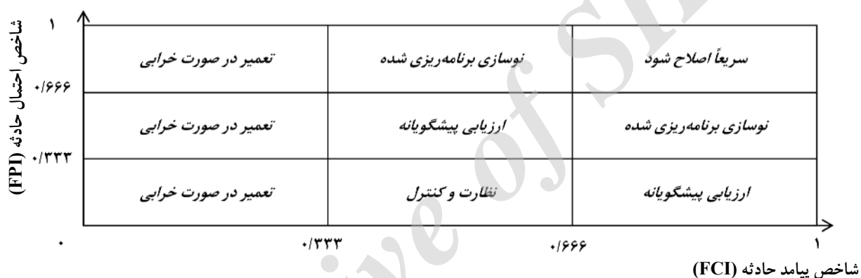
Fig. 2. Determination of pipe rehabilitation strategies using combined effect of FPI and FCI (AWWA 2014) in WDSR-Min model
