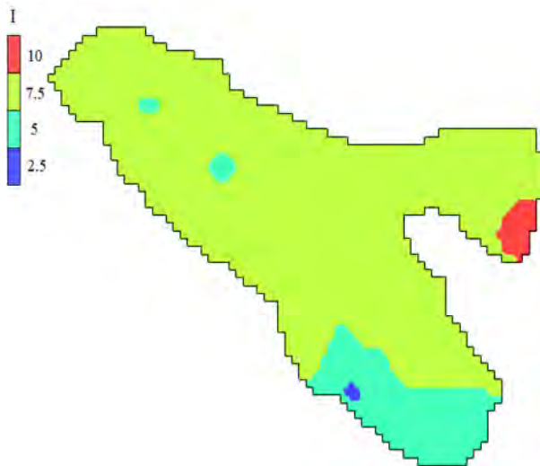
Fig. 7. Rating of parameter I (impact of the existing status of seawater intrusion) in the GALDIT model for Qom aquifer
