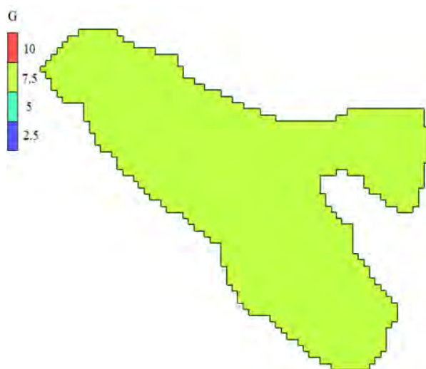
Fig. 2. Rating of parameter G (aquifer type) in the GALDIT model for Qom aquifer
