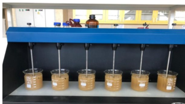
Fig. 1. A view of the Jar test to determine the optimum coagulant in the turbidity of 500 NTU
