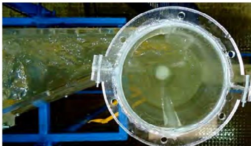
Fig. 5. The vortex flow observed at the beginning of the vertical shaft
