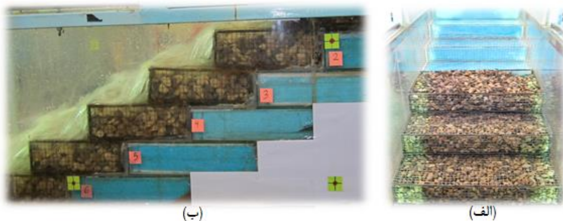
Fig. 3- Installing gabion packages on stepped spillway
