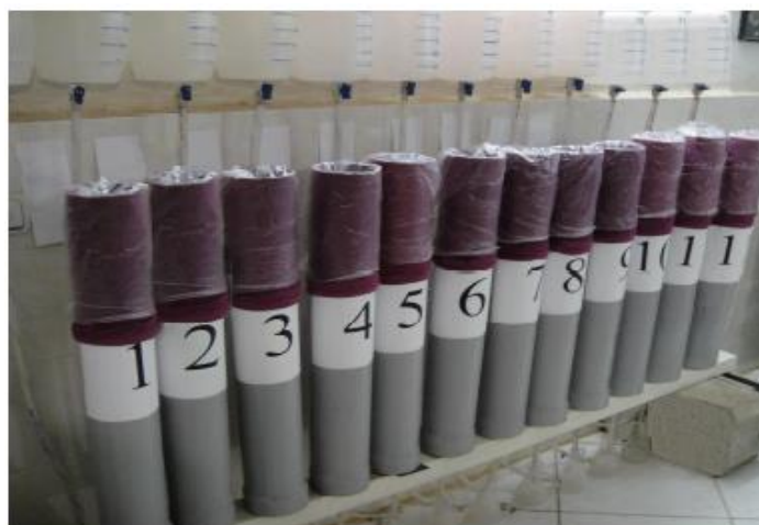
Fig. 2-Physical Designed model for desalinization and desodification
