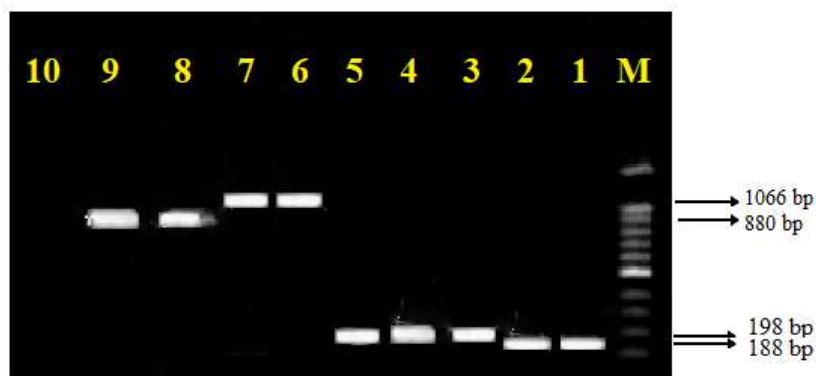
Figure 2. Electrophoresis of ica operon genes PCR products lane M -marker 100 bp, lanes 1 and 2- positive samples for icaA gene (188 bp), lanes 3 to 5- positive samples with icaD gene (198 bp), lanes 6 and 7- positive samples for icaC gene (1066 bp), lanes 8 and 9- positive samples for icaB gene (880 bp), lane 10- Negative control (distilled water)
