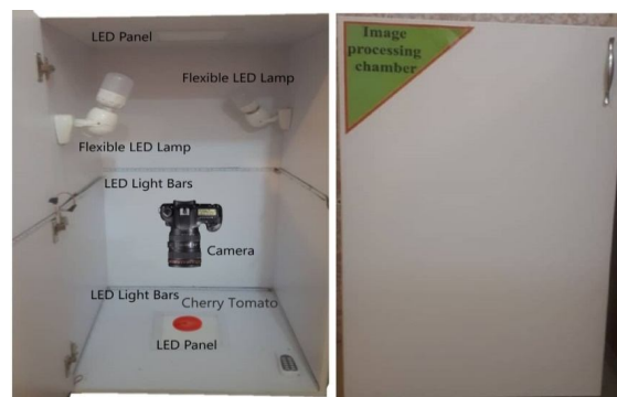
Fig 1 Scheme of Artificial vision system (AVS) set-up.
