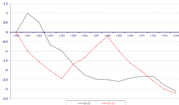
Fig. 10- My nonparametric test diagram Mann-Kendall and changes in U_i and U'_i components of static surface data of observation wells
