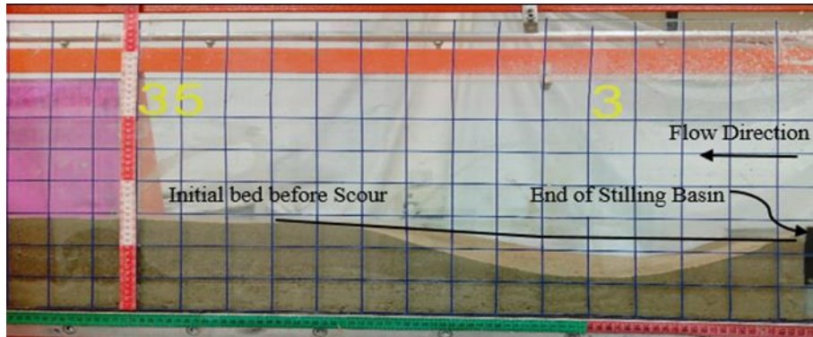
Fig. 5- Scour created in the laboratory at Froude number 2.68
