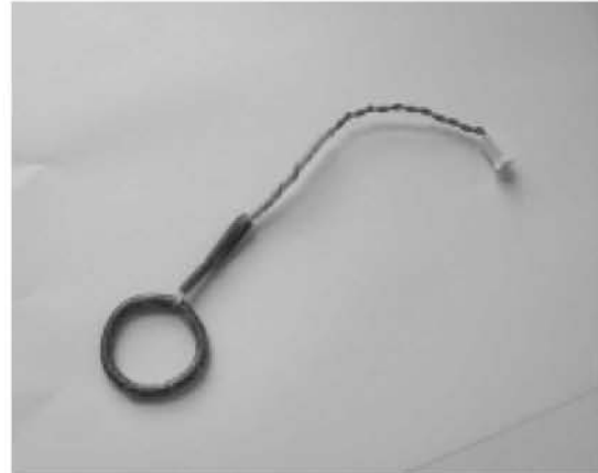
Figure-2: Rogowski coil is used for rotor bar current measurement
