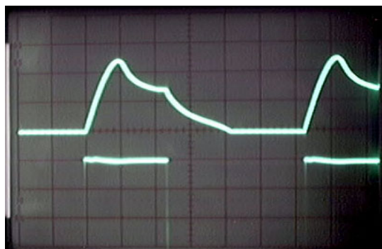
Fig. 6 a– Actual current waveforms for 14 Deg. of Advancement b– Power switches turn on time duration
