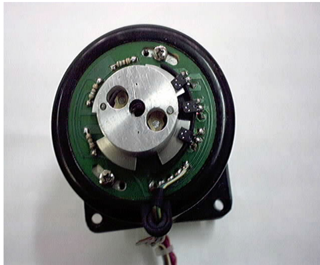
Fig. 7 The governor on the motor shaft
