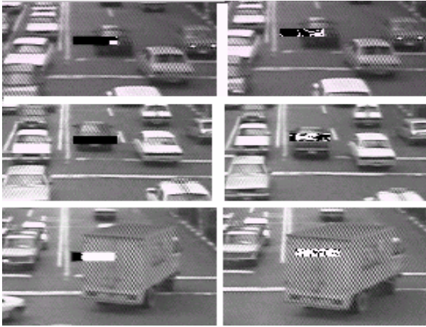
Figure 3. Left images show the edges detected with morphological operator. Right images show the result with the GR operator. Note that the edges are detected only inside the small sub-window that is visible at image center.
