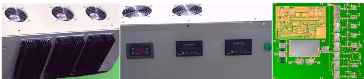
Figure .5: fuel cell test system a) rear panel B) front panel c) control board
