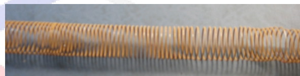
Fig. 4 Tube insert tested in experiments (wire coil Type 1)
