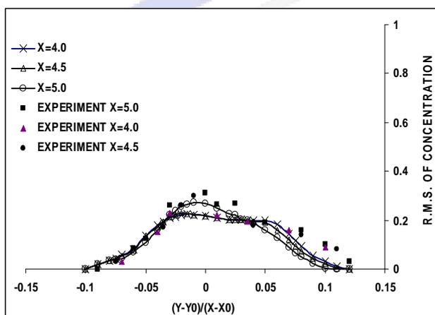
Fig(10): Time-averaged concentration fluctuations for different cross-sections and  $Pe=2500$ , comparison with Ref [8]
