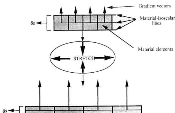
Fig(1): The relation between stretching rate of iso-scalar lines and scalar gradient
