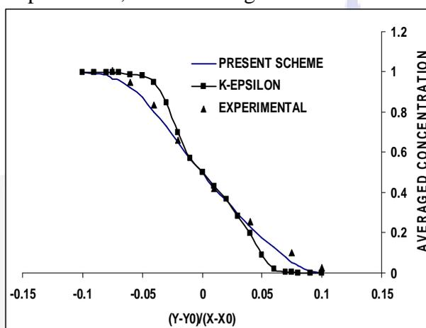
Fig(11): Time-averaged concentration profile at  $x=5$  for  $Pe=2500$  compared with other numerical method
