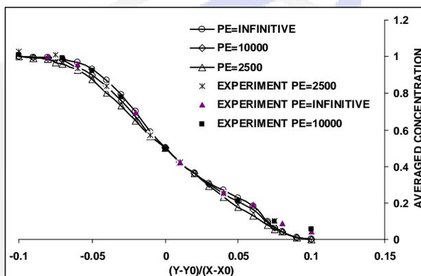
Fig(7): Time-averaged concentration profile at  $x=5$  for different Peclet numbers, comparison with Ref [8]
