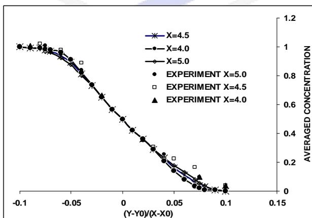
Fig(8): Time-averaged concentration profile for different cross-sections and  $Pe=2500$ , comparison with Ref [8]
