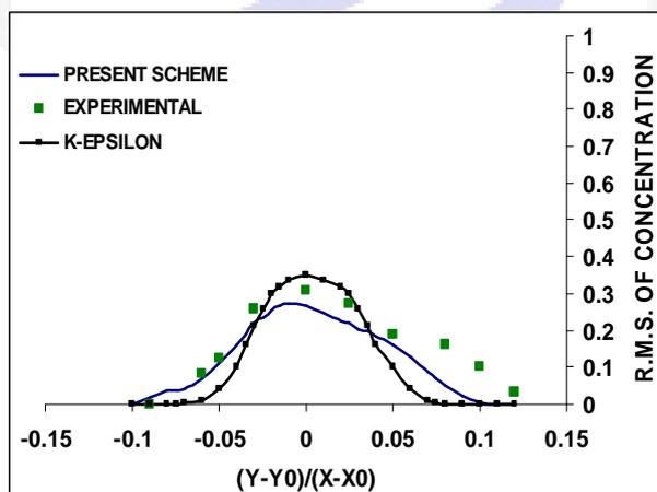
Fig(12): Time-averaged concentration fluctuations at  $x=5$  for  $Pe=2500$  compared with other numerical method
