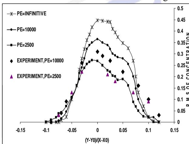
Fig(9): Time-averaged concentration fluctuations at  $x=5$  for different Peclet numbers, comparison with Ref [8]
