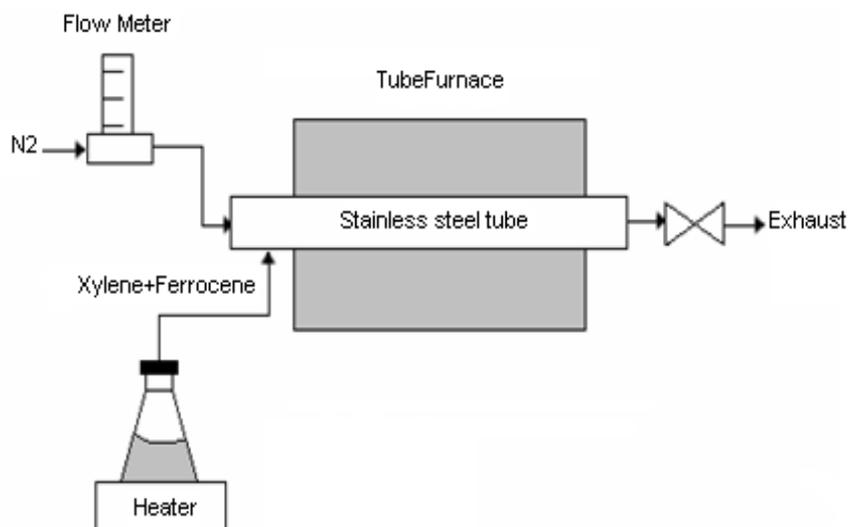
Figure 1. Schematic diagram of the experimental CVD set-up.
