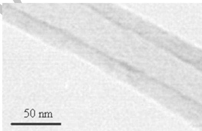
Figure 4. TEM image of purified CNTs.
