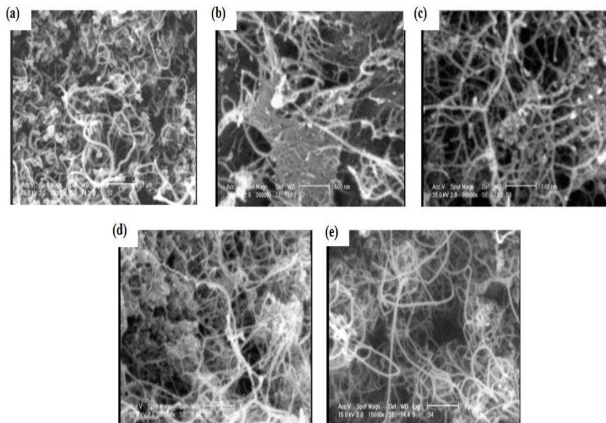
Figure 2. SEM images of (a) raw CNTs, (b) CNTs treated with HNO<sub>3</sub> /H<sub>2</sub>SO<sub>4</sub> (1/3), (c) HNO<sub>3</sub> /H<sub>2</sub>SO<sub>4</sub> (1/1), (d) HCl 8 M and (e) HNO<sub>3</sub> 8 M .
