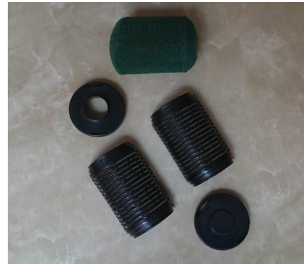
Fig. ۱۶. Components of an absorbent filter
