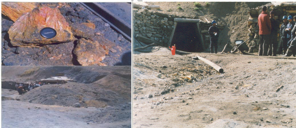
Figures 4 and 5: In Zarshuran mine, rainfall penetrates into the mining tunnels easily and it is in direct contact with wastes
