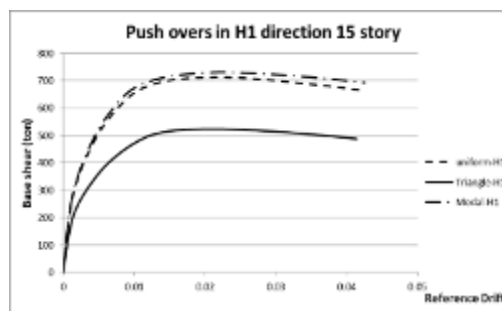
Figure 7. Comparing Modal pushover curves with uniform and triangle load distribution for the 15-story building
