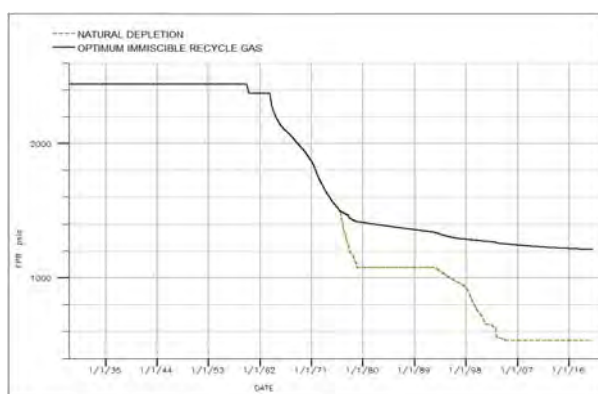
Figure 13: Average field pressure of optimum EOR condition in comparison with natural depletion.
