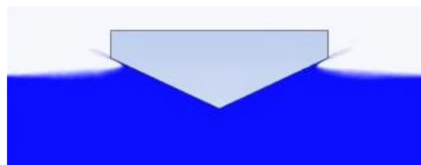
Figure 3: Free surface of liquid for impact of wedge during water entry
