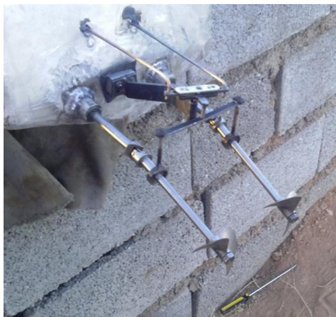
Figure 5: The moving shaft propulsion system
