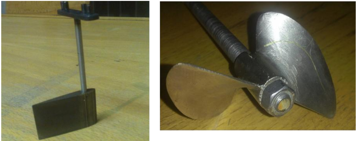
Figure 8: Propeller of the craft (right) and rudder of the craft
