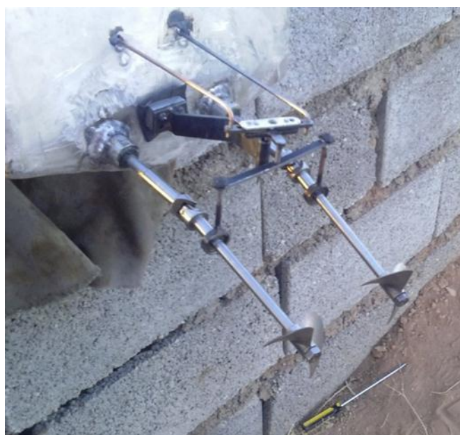
Figure 5: The moving shaft propulsion system
