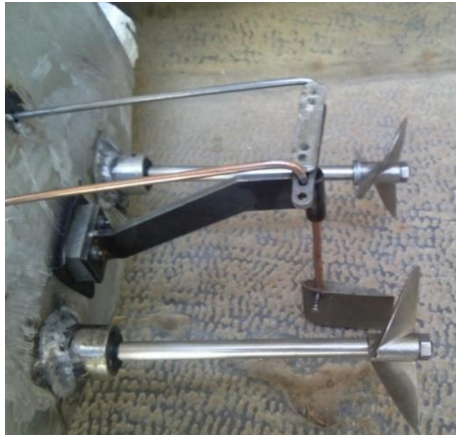
Figure 6: Propulsion system by the rudder
