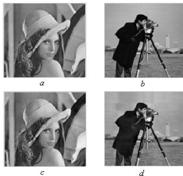
Figure 1: Importance of U, V matrices. a, b are original images. c, d are reconstructed images with exchanged S matrices.
