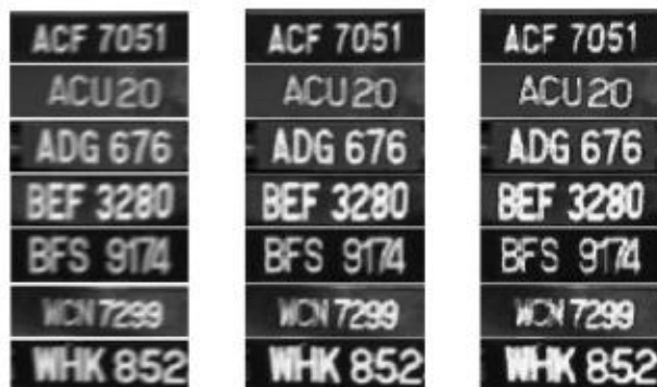
Figure 7. Final result (Left column: Input images. Two next column are output of first and second iteration of de-blurring )
