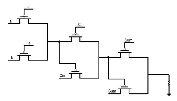
Fig4. Parity checker circuit
