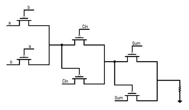
Fig4. Parity checker circuit
