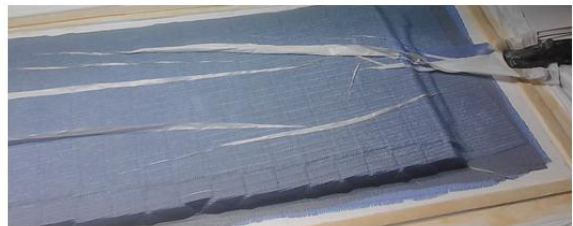
Step 3: Applying the vacuum in order to transfer resin component
