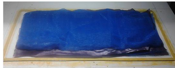
Step 2: Vacuum molding installation
