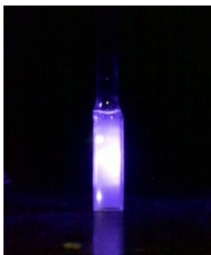
Figure 3. A photograph of white light generation by GaN-UV LED CdSe/ZnS core-shell solution
