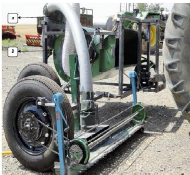
Fig. 1. Conveing system (a: cyclone, b: suction fan)[5].
