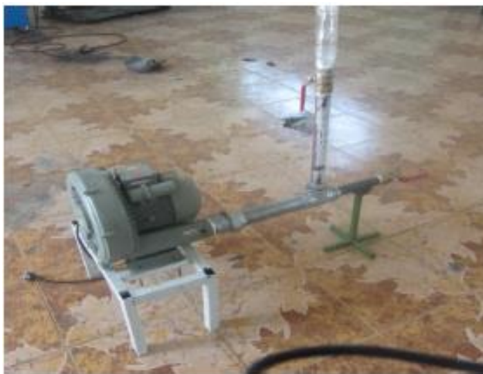
Fig.3. The wind column for measure of terminal velocity.
