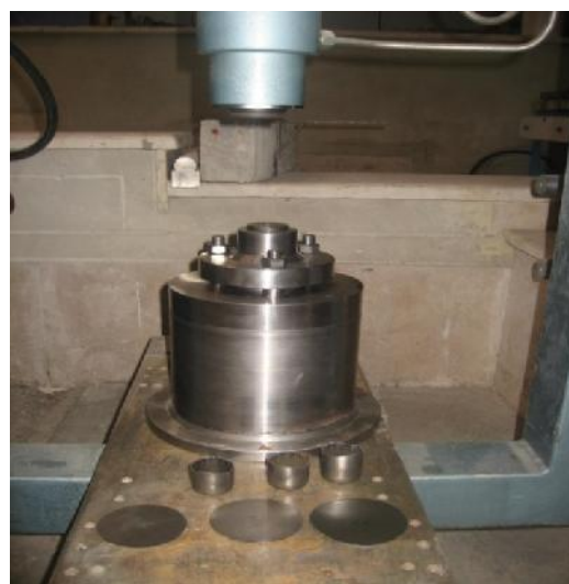
Fig. 1: Experimental deep drawing setup
