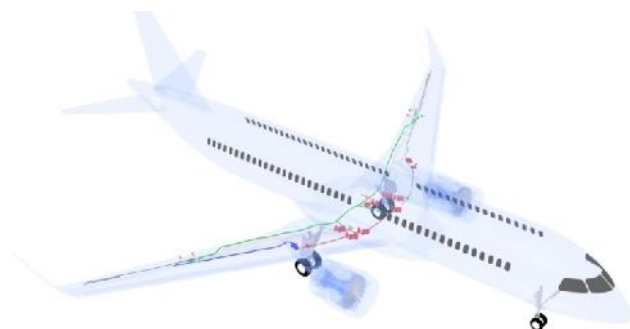
Fig. 1: J150+ civil aircraft and the fuel system located in the model.
